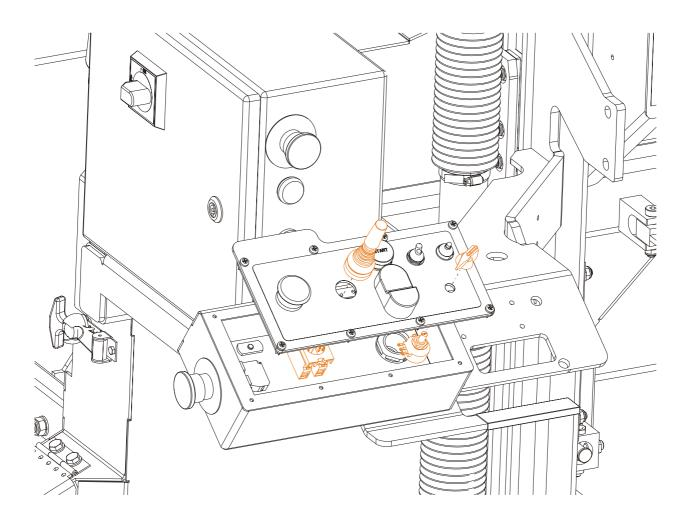
7. Mount power feed support plates with rubber bushings (2) to pins placed in the middle of bed extensions (1), screw tensioners (3) to extreme pins. Fasten spring to short tensioner.
