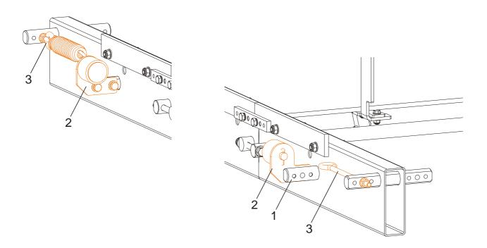
8. Mount the motoreducer with four bolts.
