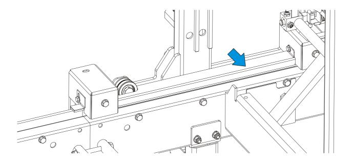
**3.** Take the rope off and remove front & rear rope mount brackets.
