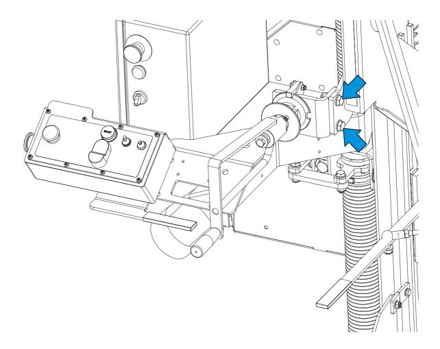
**5.** Remove the rope guide roller system.
