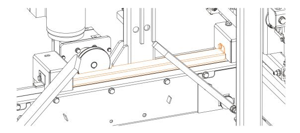
12. Mount a motoreducer pulley front cover.
