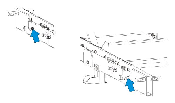
4. Remove feed crank and manual feed system support.
